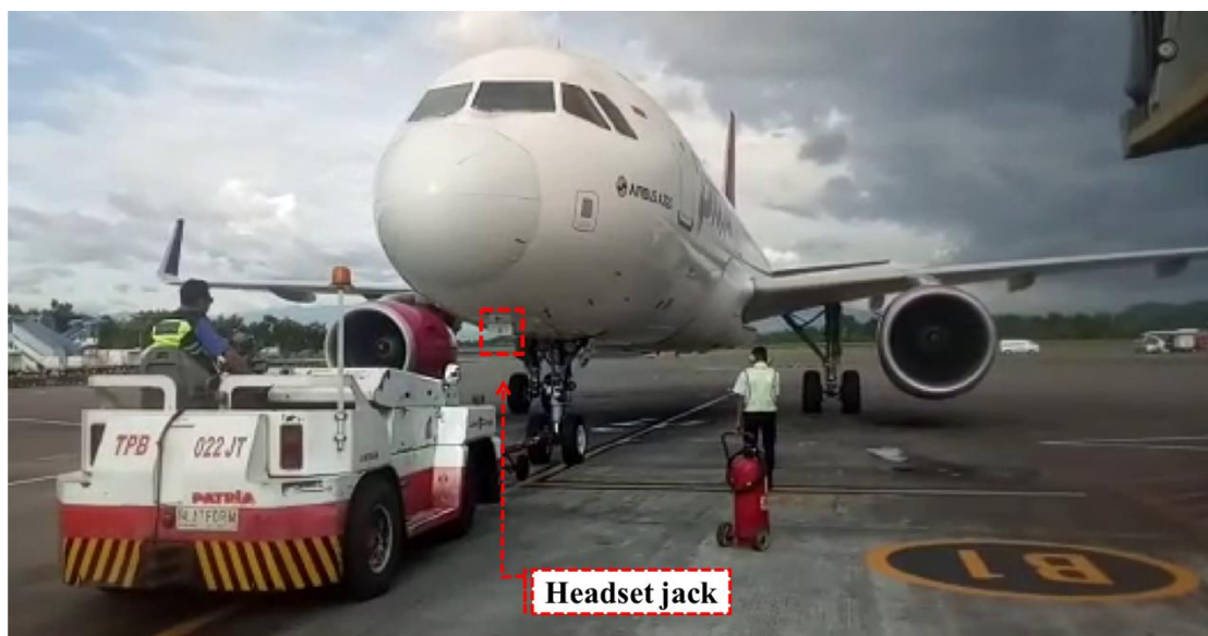
Figure 1: The common push back activity and the location of headset jack on typical Airbus A320
